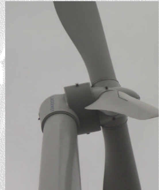
Gearless design (Zephyros & Enercon)
